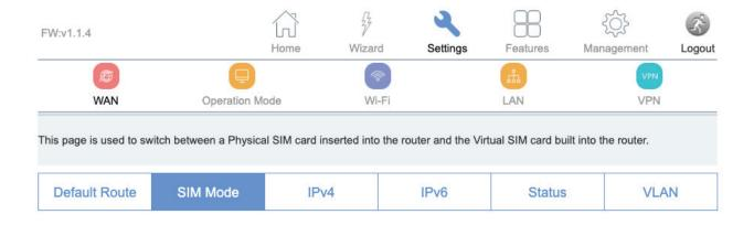
The **SIM Mode** page is used a toggle between a Physical SIM inserted in the router for internet and a Virtual built into the router for internet.
