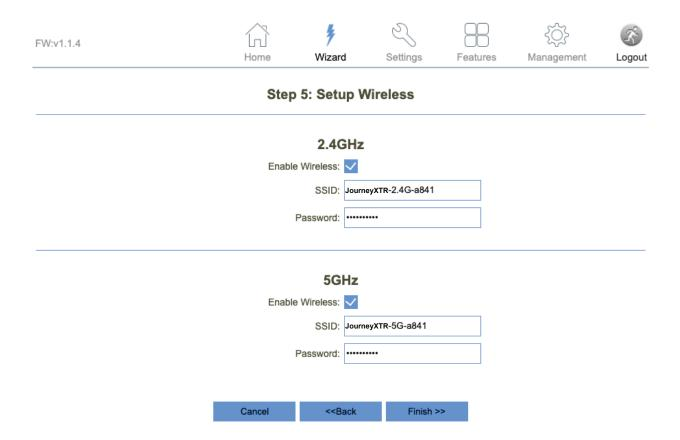
The **Setup Wireless** page is used to set the SSID and password for both the 2.4GHz and 5GHz Wi-Fi networks.
