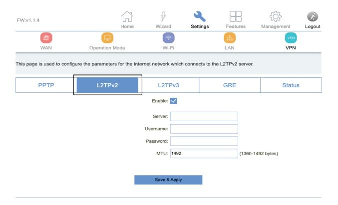
The **L2TPv2** page is used to configure the parameters for the internet network which connects to the L2TPv2 server.
